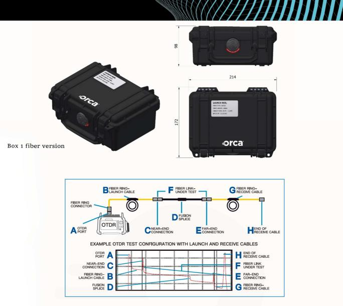
Use the Fiber Ring as a launch cable; connect the Fiber Ring between your OTDR and the fiber link under test. This will allow you to measure the loss of the near-end connection.
