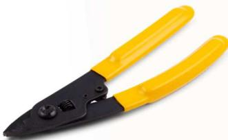
This Miller Fiber Optic Stripper is an exceptional fiber optic stripping tool that enables you to easily strip 250µm coated loose tube fiber and 900µm buffer tube. This Fiber Optic Stripping tool has hardened stripping jaws, ensuring a smooth, clean stripping action. The Fiber Optic Miller Stripper features a .0055" (0.14mm) laser drilled hole. The cushioned handle grips provide you with comfort and better control of the tool during the fiber optic stripping process.
