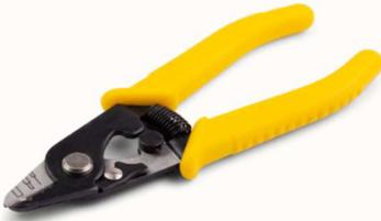
This Fiber Optic Stripper is an exceptional fiber optic stripping tool that enables you to easily strip 3mm, 250µm coated loose tube fiber and 900µm buffer tube. This Fiber Optic Stripping tool has hardened stripping jaws, ensuring a smooth, clean stripping action. The Fiber Optic Stripper features a .0055" (0.14mm) laser drilled hole. The cushioned handle grips provide you with comfort and better control of the tool during the fiber optic stripping process.
