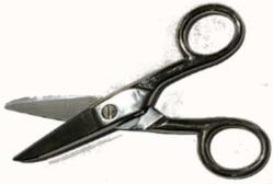
When cutting Kevlar®, you need a cutting tool with very durable blades. You also want the tool to cut cleanly, and to fit comfortably in your hand.
